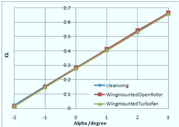
Fig.12 CL-AoA of wing mounted config
