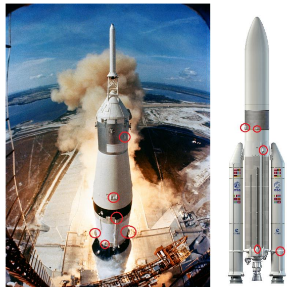
Fig 1: Examples of wedge like fairings on the Saturn V and Ariane V launch vehicles (NASA / ESA).
