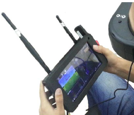
Fig. 6. Ground station hardware.
