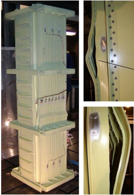
Fig. 9 – Wing stringer panel static test result
