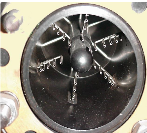
Fig. 3. Pressure rake to measure total pressure PT2 at AIP.
