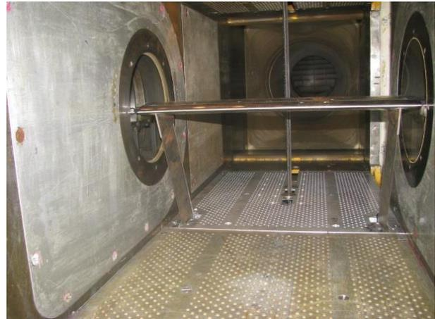
Fig. 9. T-112 TsAGI transonic wind tunnel with the model; view from the leading edge.
