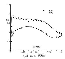
Fig. 3 Wing surface Cp comparison at Ma=0.75.
