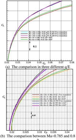
Fig. 10 Lift-to-drag characteristics comparison from ETW test data.
