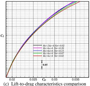
Fig. 7 Aerodynamics comparison at Ma=0.785, Re= $4 \times 10^6$  in different transition locations.
