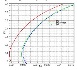
Fig. 4 Lift-to-drag characteristics comparison at Ma=0.75.
