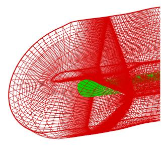
Fig. 2 DLR-F6 wing-body/nacelle grid.
