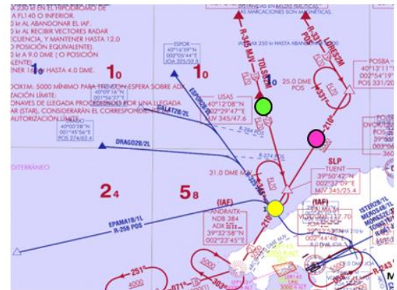
Fig. 10. Location of conflict point (yellow) between CCO and arrival flow at Palma TMA. The green and pink circles indicate the new initial points for arrivals with departing preference.
