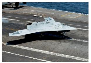
Fig. 1. Northrop Grumman X-47B UCAV
