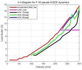
Fig. 3. V-n Diagram for F-16 Pseudo 6-DOF Model
