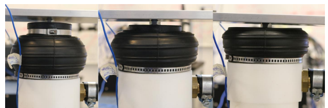
Fig 17. Air-springs at the nominal (left), reduced (center) and low (right) pressure level.
