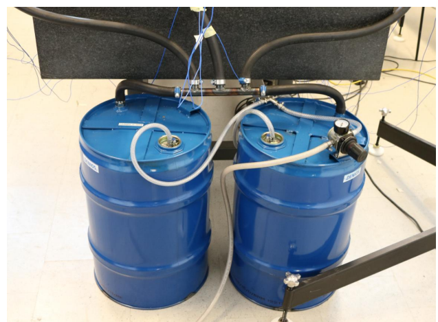
Fig 2. The two-barrel pressure vessel for the air-spring support system.
