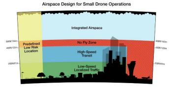
Fig. 5. Amazon proposal for airspace design for small drone operations [17]
