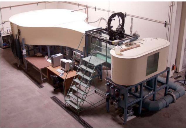
Fig. 2 The RHRC water tunnel model 2436
