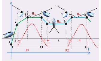
1-2 take-off & rise; 2-3 first climb; 3-4 first cruise; 4-5 descent; 5-6 hovering in the night; 6-7 climb; 7-8 cruise in the daytime Fig.8 Flight Profile of Ladder
