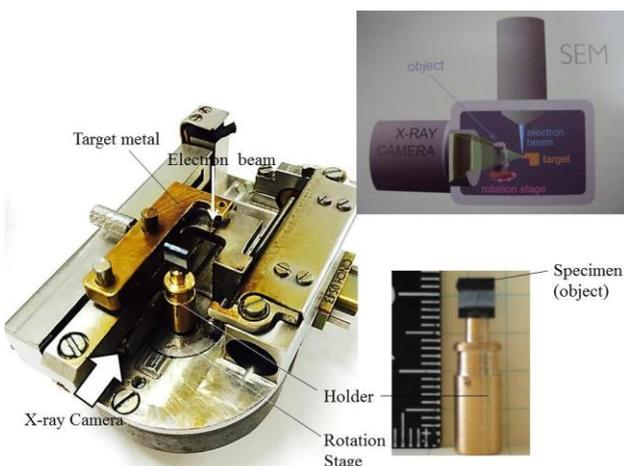
Fig.2 Specimen on a metal holer
