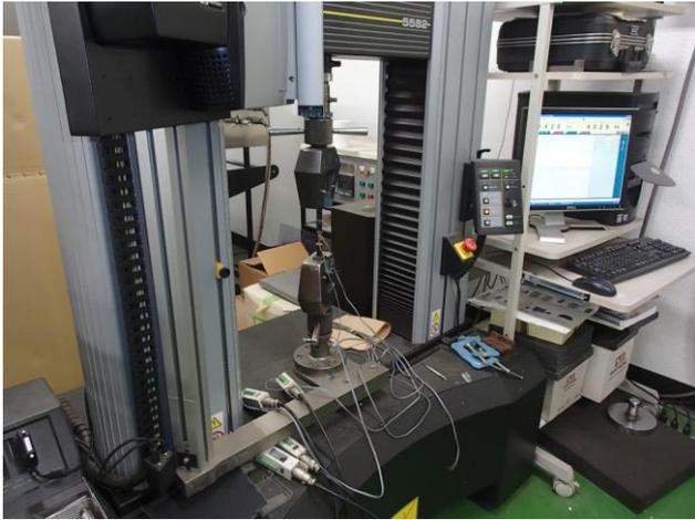
Fig.4 Tensile test on CF3 sample
