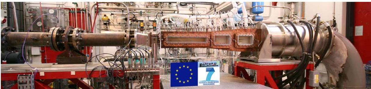
Fig.8 LAPCAT2 supersonic combustor in LAERTE Facility
