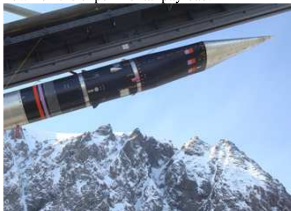
Figure 4 The HIFiRE-5 elliptic cone boundary layer transition experiment payload ready for flight.
