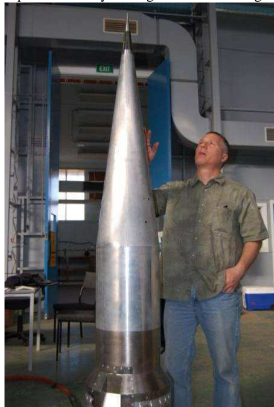
Figure 3 The HIFiRE-1 cone boundary layer transition experiment payload ready for flight.
