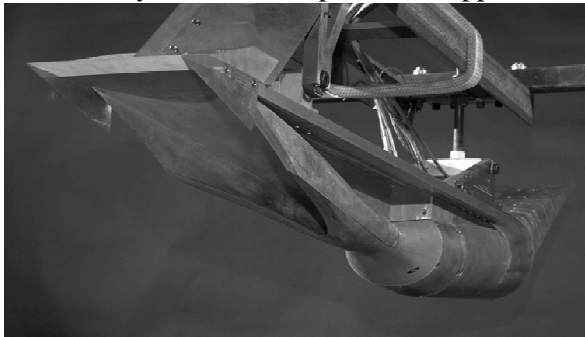
Figure 8 A scramjet engine employing a REST inlet as tested in the T4 shock tunnel.
