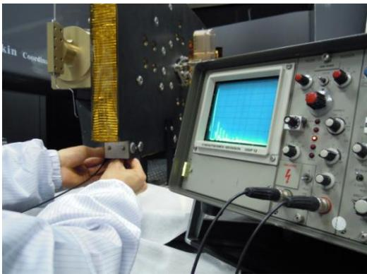
Fig. 24. Ultrasonic Inspection of bonding layer
