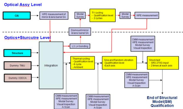
Fig. 13 Qualification Test Flow with SM
