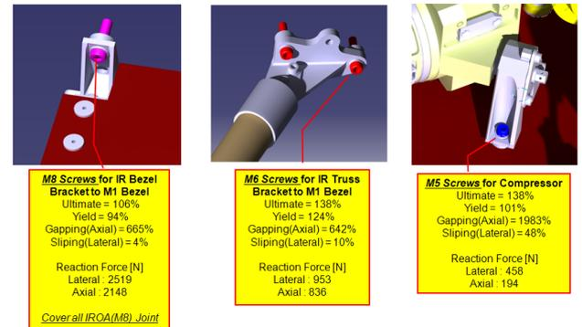
Fig. 7. MoS summary of joint screws by design load 25g
