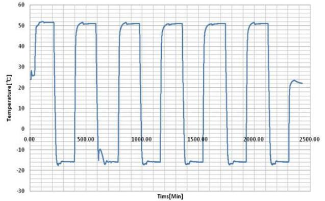
Fig. 21 Thermal cycle test profile
