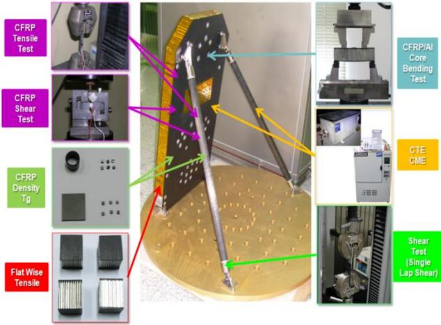
Fig. 3. Coupon test location
