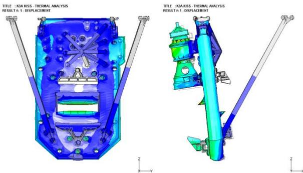
Fig. 12. Example of distortion analysis with 12K uniform temperature change
