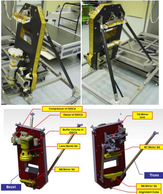
Fig. 2. Configuration of Structure
