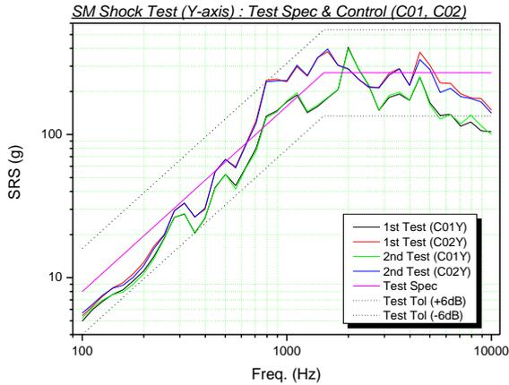
Fig. 19. Shock test profile and CG response.
