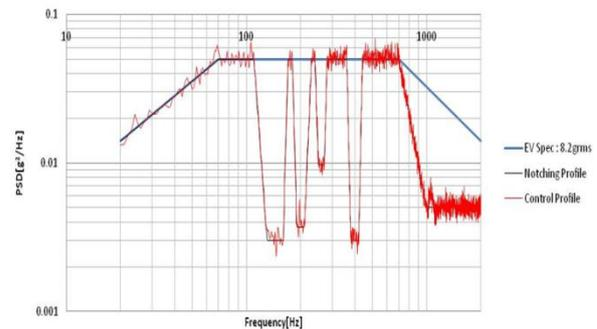
Fig. 17. Random vibration test profile of X-axis (Specification vs. Notching Ref. vs. Controlled)
