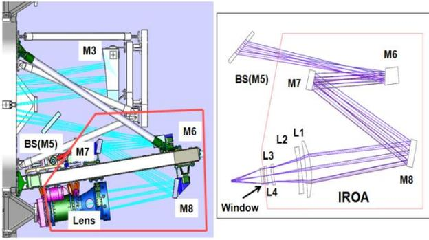
Fig. 1. Optical Design Layout
