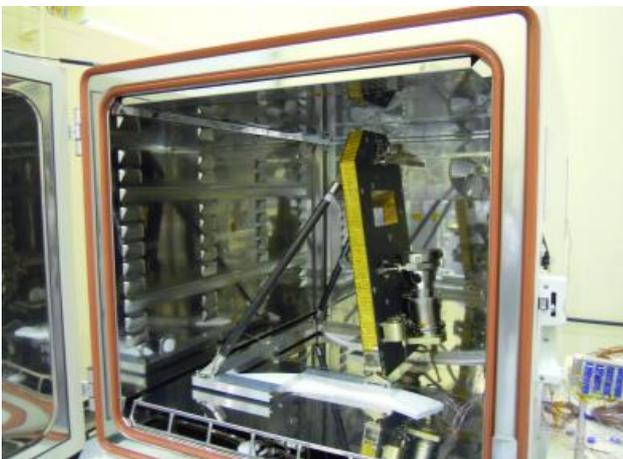
Fig. 20 Thermal cycle test configuration in TCT chamber with MGSE
