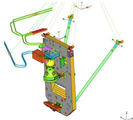
Fig. 4. Finite Element Model
