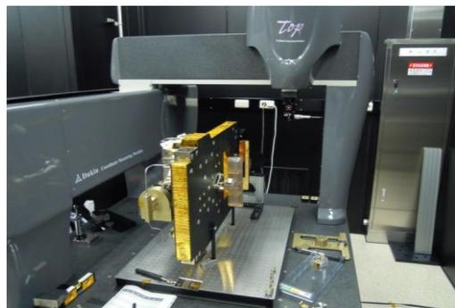
Fig. 22. 3D dimension measurement
