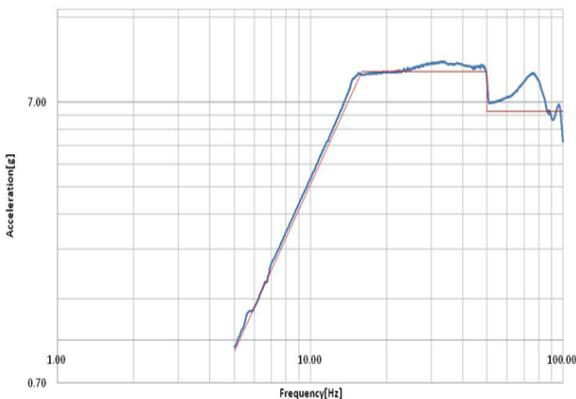
Fig. 16. Sine vibration test profile and CG response (ex. Z-axis)
