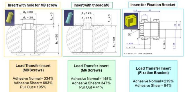
Fig. 8. MoS of inserts bonding parts by design load 25g
