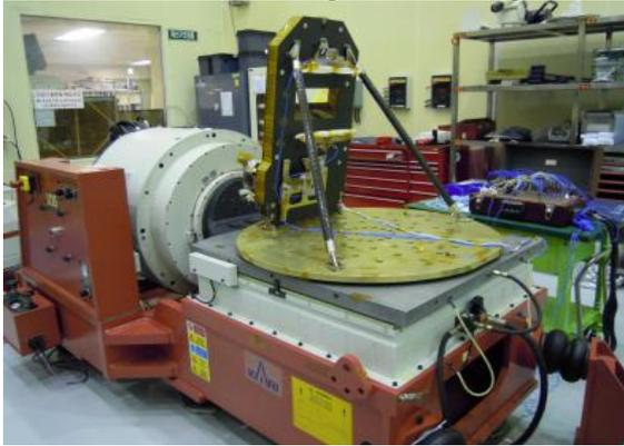
Fig. 14. Vibration test configuration (ex. X-axis)
