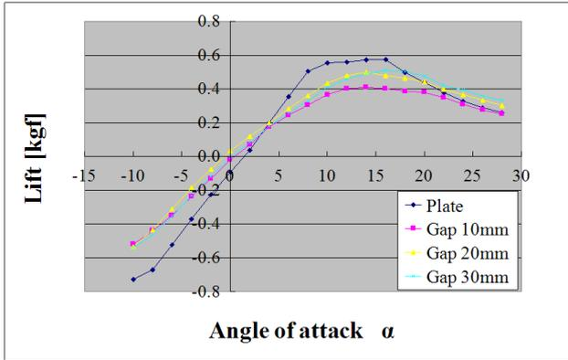
Fig. 11. Lift vs.  $\alpha$  ( $V=15\text{m/s}$ )
