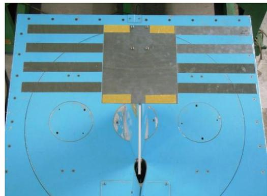
Fig. 6. Wing with 30mm gap
