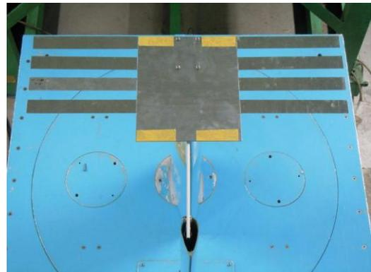
Fig. 5. Wing with 20mm gap
