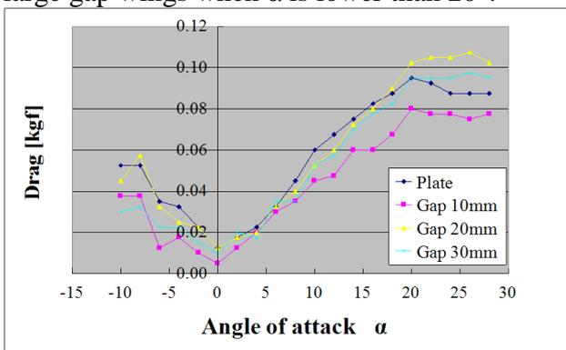
Fig. 8. Drag vs.  $\alpha$  ( $V=10\text{m/s}$ )
