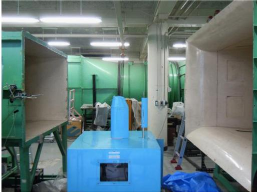
Fig. 7. Low-speed Göttingen type wind tunnel
