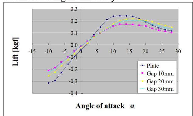
Fig. 10. Lift vs.  $\alpha$  ( $V=10\text{m/s}$ )
