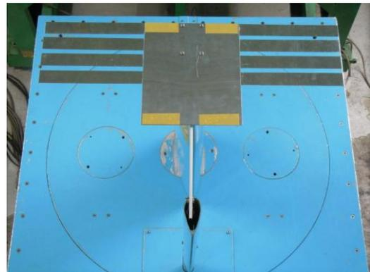
Fig. 4. Wing with 10mm gap
