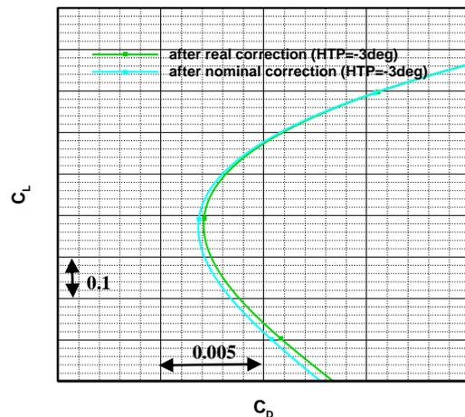
Fig. 13. Drag polar after real correction and nominal correction for configurations with -3 degree HTP deflection
