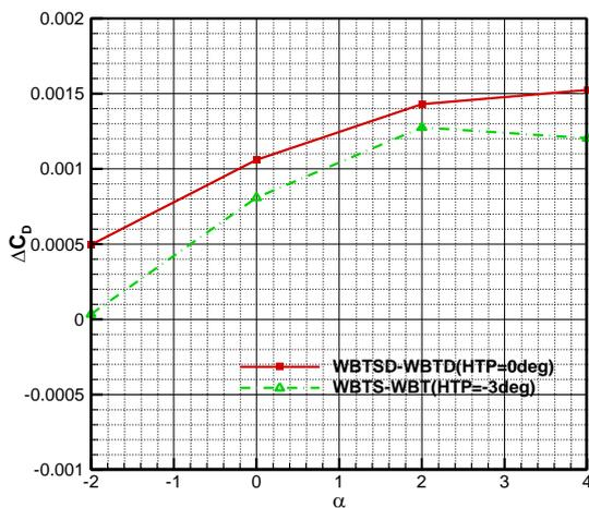
Fig. 11. Nominal and real correction on drag coefficients for configurations with -3 degree HTP deflection
