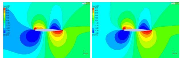
Fig. 9. Comparison of the local angle of attack on a cross-section plane of HTP
