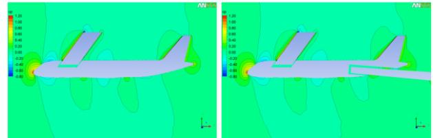
Fig. 8. Comparison of the pressure coefficient on the symmetry plane
