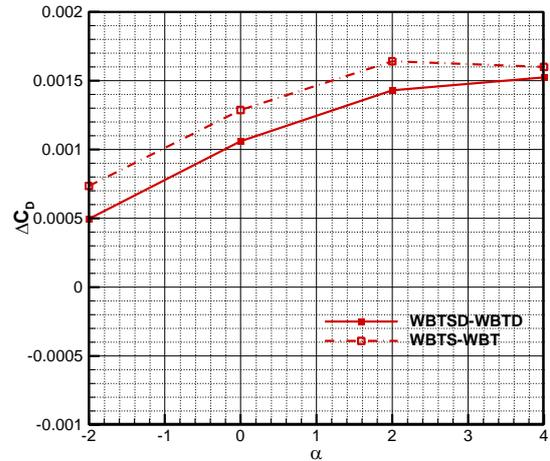
Fig. 4. Real and nominal rear sting interference correction on drag coefficients
