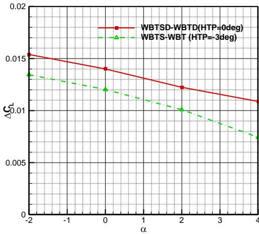
Fig. 10. Nominal and real correction on lift coefficients for configurations with -3 degree HTP deflection
