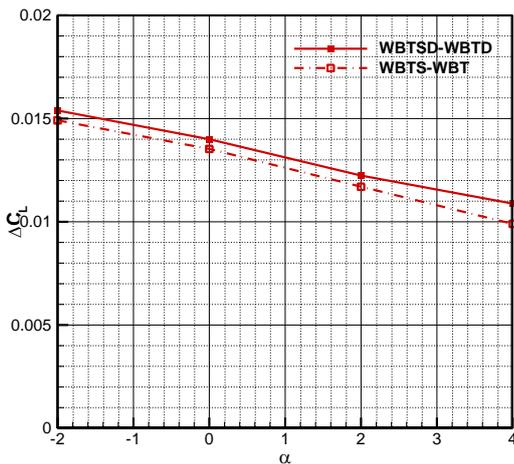
Fig. 3. Real and nominal rear sting interference correction on lift coefficients
