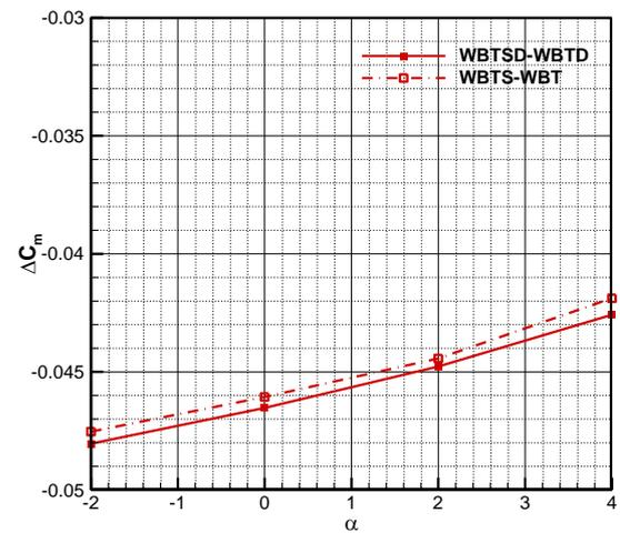
Fig. 5. Real and nominal rear sting interference correction on pitching moment coefficients
