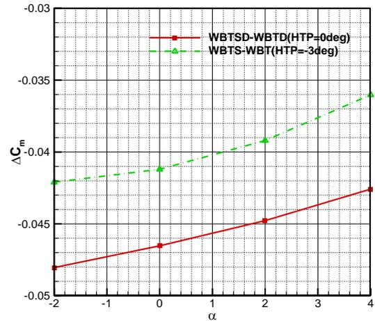
Fig. 12. Nominal and real correction on pitching moment for configurations with -3 degree HTP deflection
