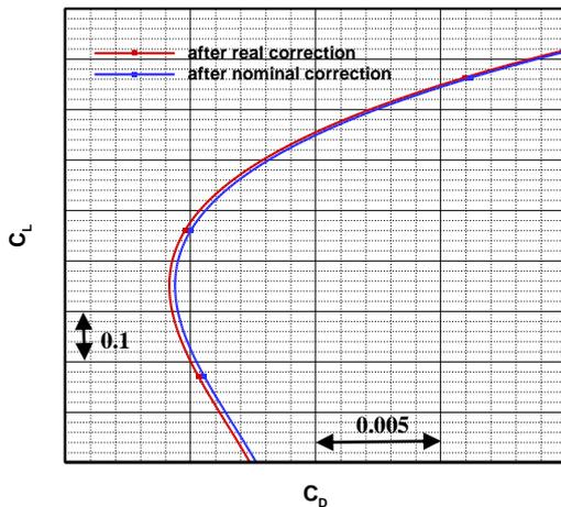
Fig. 6. Drag polar after real correction and nominal correction
