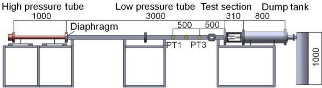
Fig. 1. Shock Tunnel. (unit: mm)
