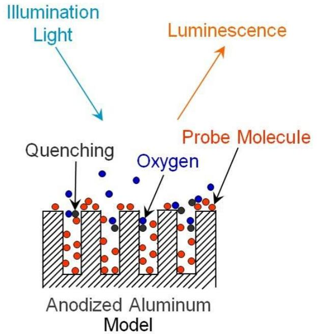
Fig. 5. Schematic diagram of AA-PSP structure.
