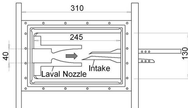
Fig. 2. Test Section. (unit: mm)
