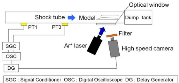
Fig. 6. Schematic diagram of PSP system.
