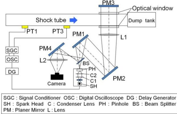
Fig. 4. Schematic diagram of shadowgraph system.
