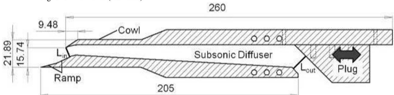
Fig. 3. Supersonic Intake model. (unit: mm)
