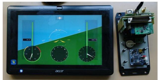
Fig. 13. EFIS Running on Acer Iconia Tab Windows7 with Disassembled AHRS unit
