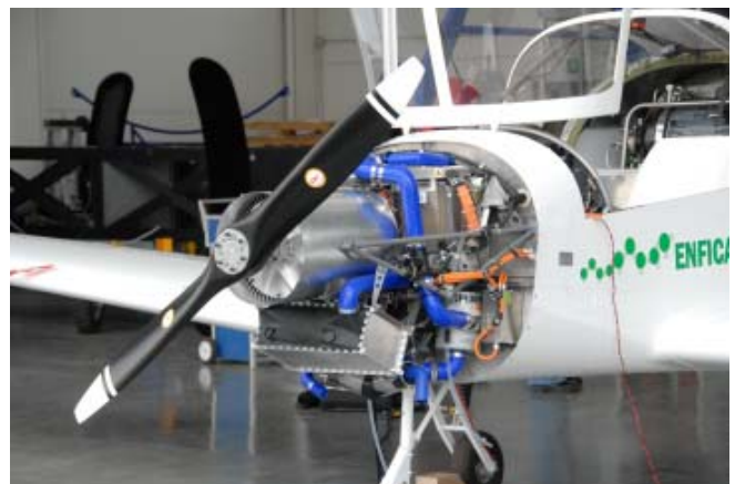
Fig. 3. Engine bay instalments of the fuel cell.
