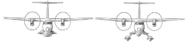
Fig. 4: Retracting Float Concept [9]
