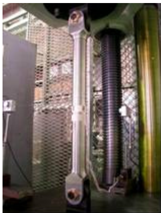
Fig. 7 Compression Test of TiMMC Side Stay
