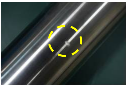
Fig. 16 Indication after 40 joules Impact Test
