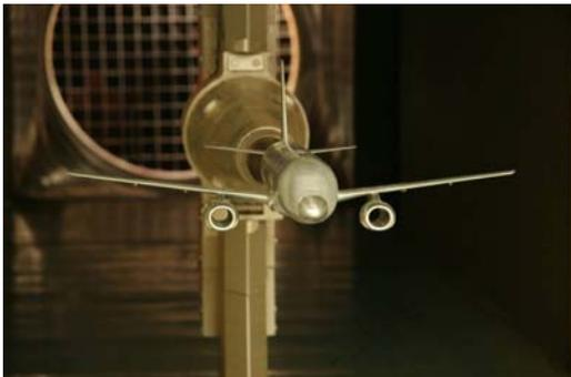
T-128 transonic wind tunnel testing
