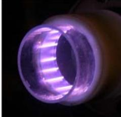
New concept based on direct control of noise radiation mechanisms by plasma actuators (DBD)
