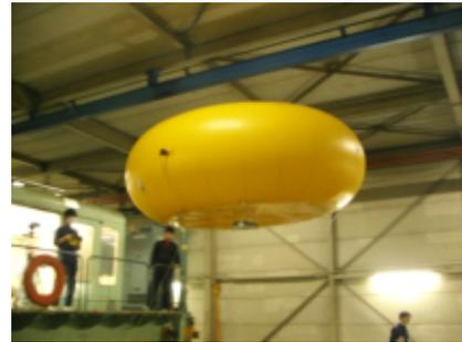
Fig. 17. Model for free-flight with propulsion device (small black point on the side)
