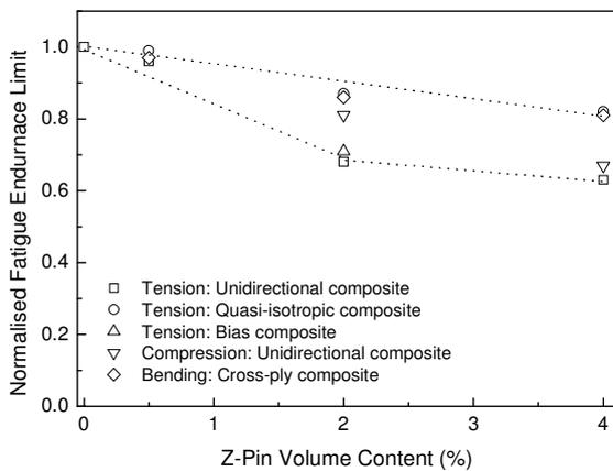
Fig. 10. Effect of z-pin content on normalised fatigue endurance limit of carbon-epoxy.
