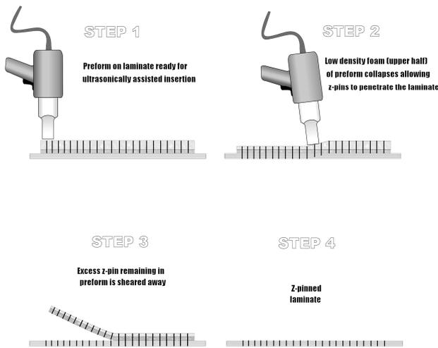
Fig. 1. Major stages in the insertion of z-pins into uncured composite material.
