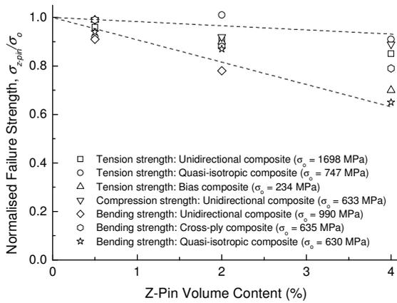
Fig. 7. Effect of z-pin content on the normalised failure strength of carbon-epoxy.
