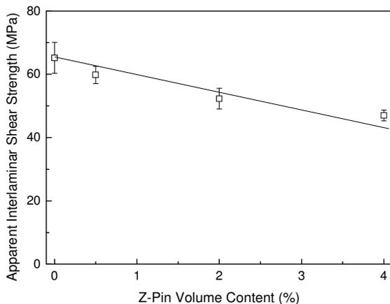
Fig. 11. Effect of z-pin content on the apparent interlaminar shear strength of cross-ply carbon-epoxy.
