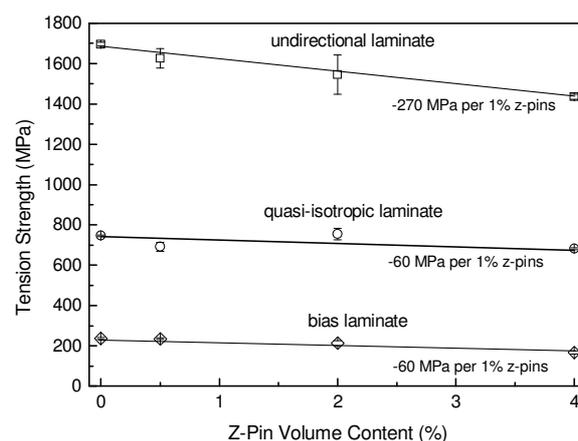
Fig. 6. Effect of z-pin content on the tension strength of carbon-epoxy.
