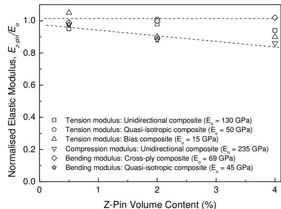
Fig. 4. Effect of z-pin content on the normalised elastic modulus of carbon-epoxy.
