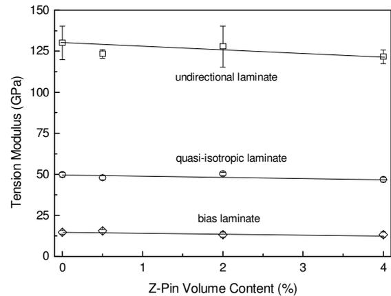
Fig. 3. Effect of z-pin content on the tension modulus of carbon-epoxy.
