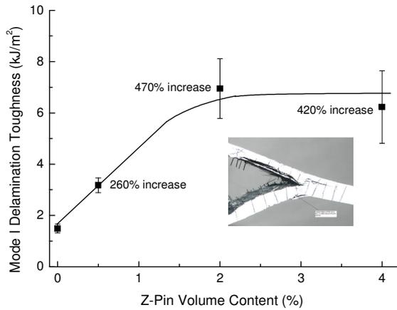
Fig. 2. Effect of percentage volume content of z-pins on the mode I interlaminar toughness.
