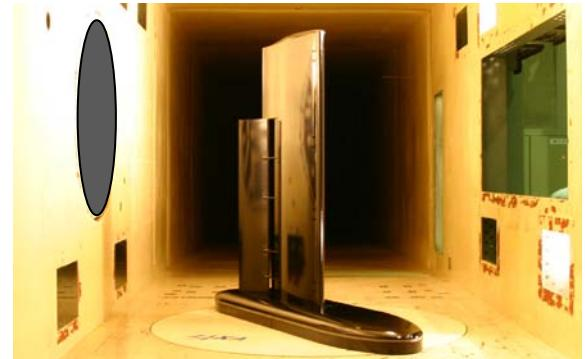
Fig. 3 JAXA LWT2 hard wall test section
