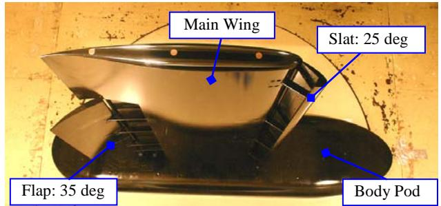
Fig. 1 Simplified High-Lift Model
