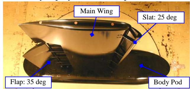
Fig. 1 Simplified High-Lift Model
