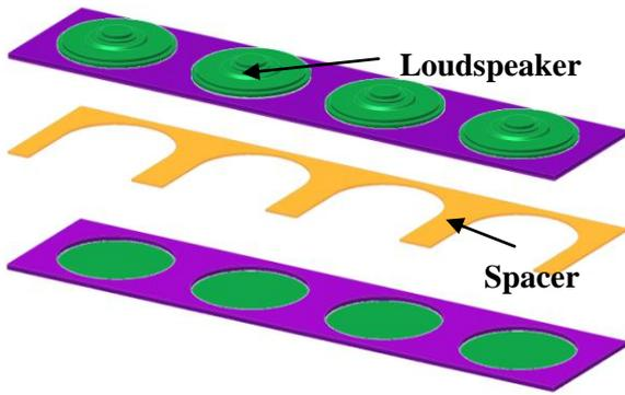
Fig. 1 The synthetic jet actuator
