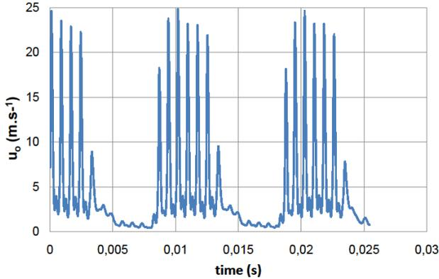
Fig. 2 Magnitude of instantaneous slot output velocity  $u_o$ , exciting frequency  $f_c = 1290$  Hz and  $f_{AM} = 100$  Hz, Actuator 1.
