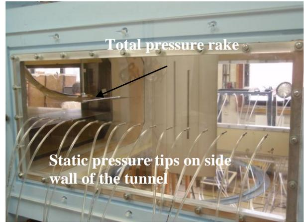
Fig. 3 Position of the model in wind tunnel
