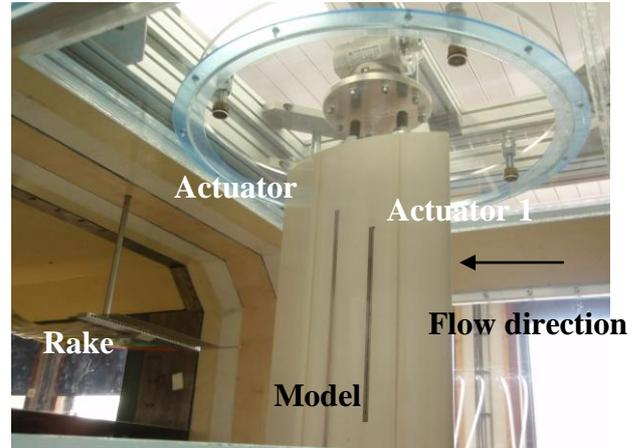
Fig. 4 Position of the actuators on the model
