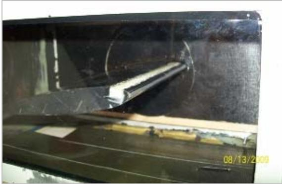
Fig. 8. Dynamic roughness wind tunnel model.
