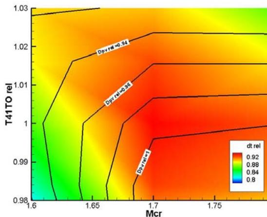
Fig. 3. Influence of  $T41TO$  and  $M_{cr}$  on emission parameters  $D_{pv,rel}$  and  $dt_{rel}$ .
