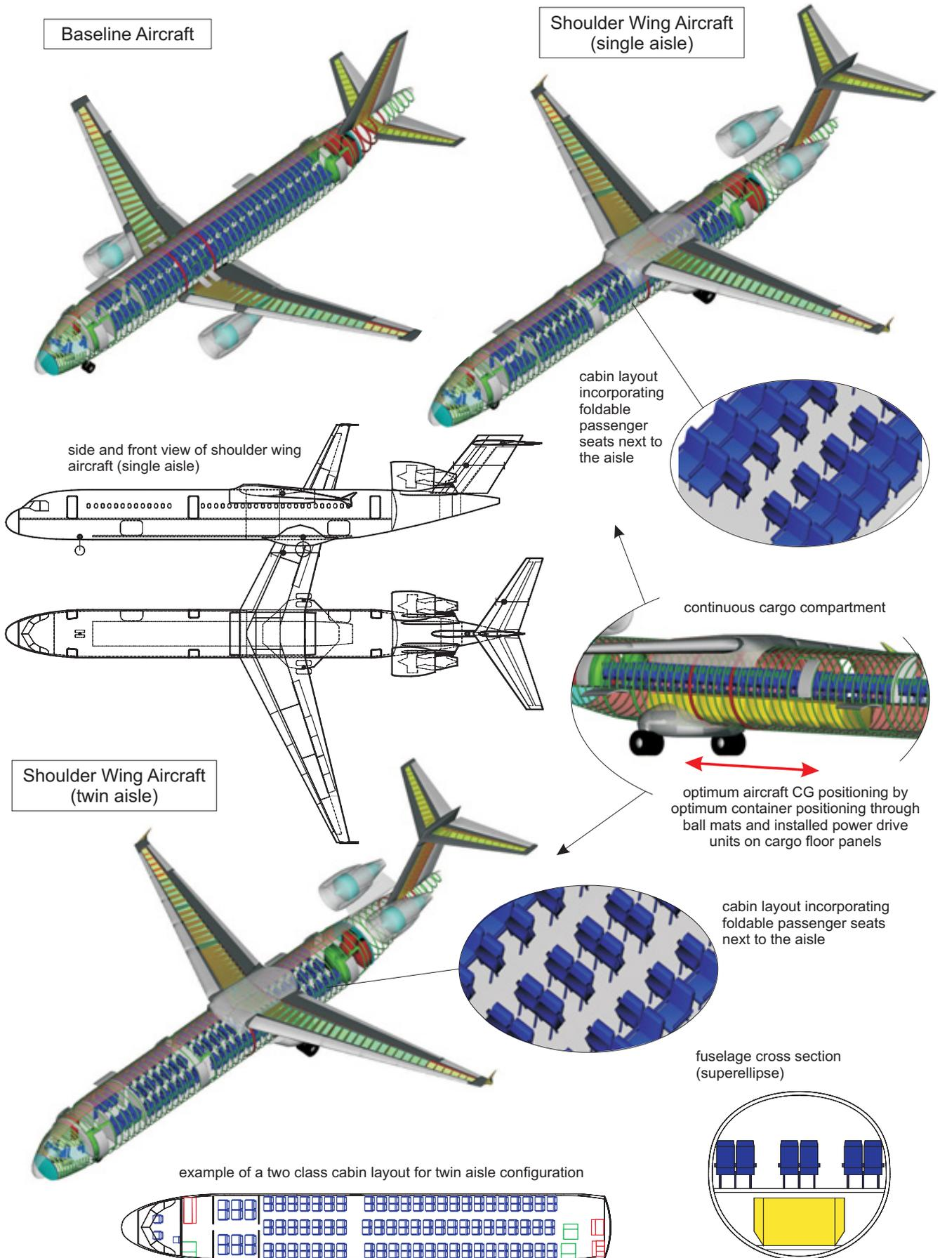
**Fig. 6** PrADO 3D visualization using Tecplot of baseline aircraft (top left), single aisle shoulder aircraft (top right), and twin aisle shoulder wing aircraft (not further investigated in terms of ground handling).
