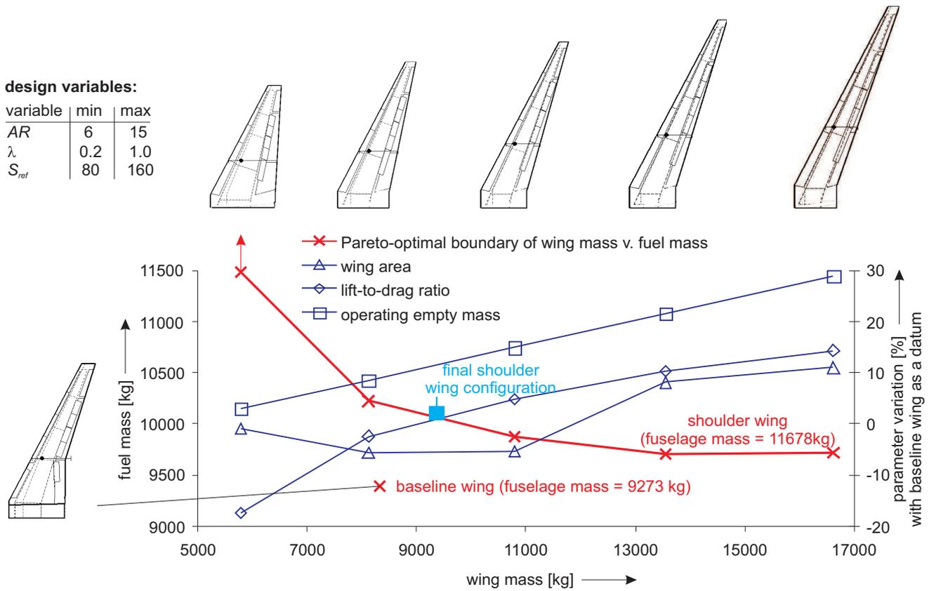
**Fig. 4** Pareto optimal boundary of min. wing mass v. min. fuel mass of the shoulder wing (red curve) vs. the baseline wing (red cross); note that the top left point could even be at higher fuel masses because the optimization at this point was restricted by the preselected aspect ratio lower limit of  $AR = 6$ .
