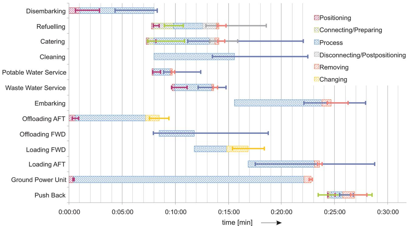
**Fig. 5** Turnaround Gantt chart of ground handling scenario I of the baseline aircraft [22]: process bars scaled according to regression analyses, lines represent standard deviations out of statistical evaluations
