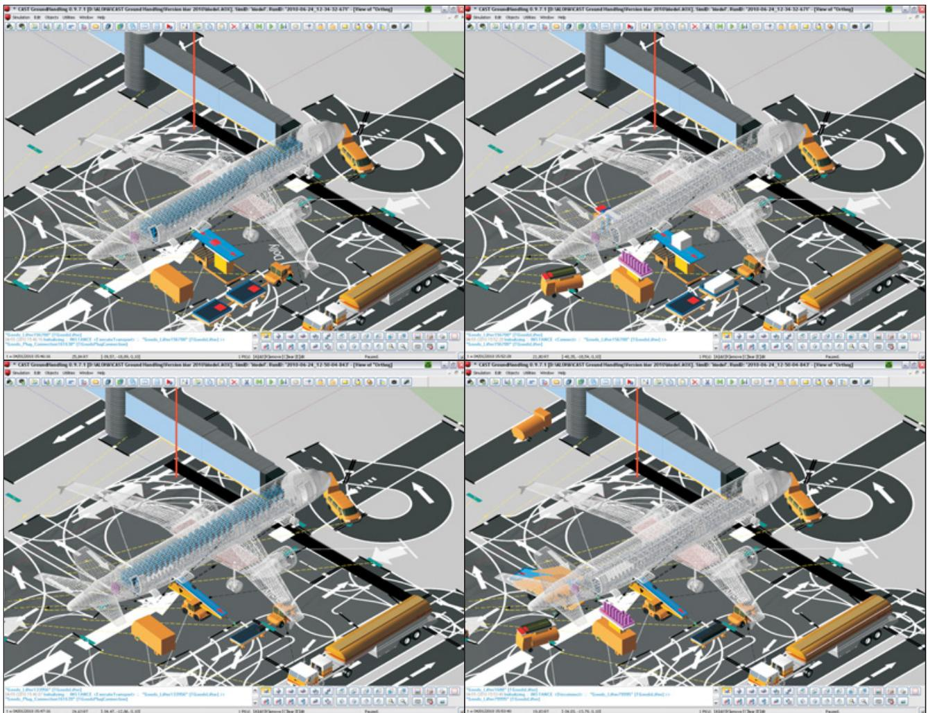
**Fig. 7** Turnaround simulation with CAST Ground Handling at different time stamps of the baseline aircraft (3D geometry out of PRADO): ground handling scenario I at the top (left 04:45, right 10:57), scenario III at the bottom (left 05:45, right 12:09); left: PAX disembarking; right: all PAX disembarked. Turnaround simulation of adapted aircraft designs is still in progress.
