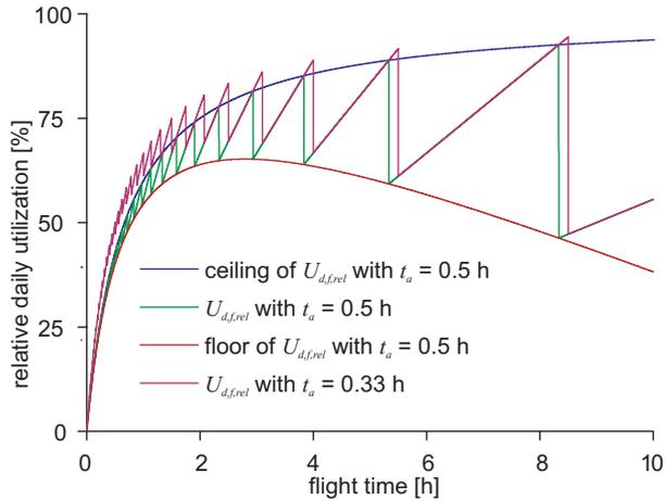
**Fig. 2**  $U_{d,f,rel}$  over  $t_f$  at different  $t_a$  with  $A_d = 18$  h,  $t_t = 10$  min
