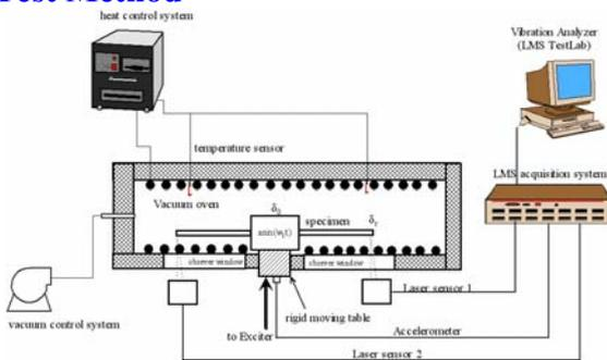
Fig 1 Material damping measuring scheme basing on a resonance dwell technique
