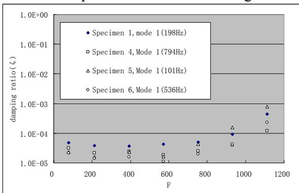
Fig. 6 Damping test result of Ti-6-4
