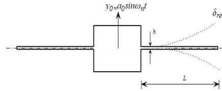
Fig 2 Double reed cantilever sample excited by base motion
