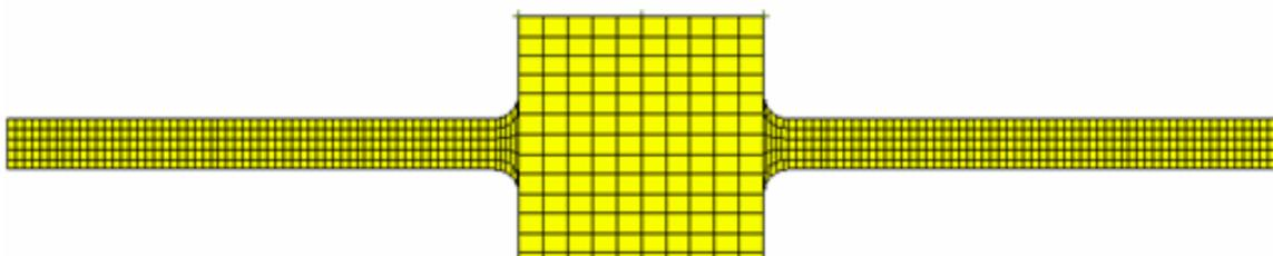
Fig.4 Finite element model of a double reed specimen
