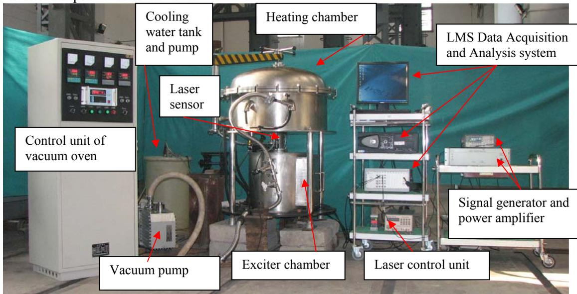
Fig 3 High temperature material damping measurement system
