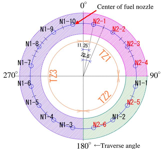
Fig.3. Schematic drawing of fuel nozzle allocation and segmentation of traverse zone into TZ1, TZ2 and TZ3. (Viewing from downstream of combustor exit.)
