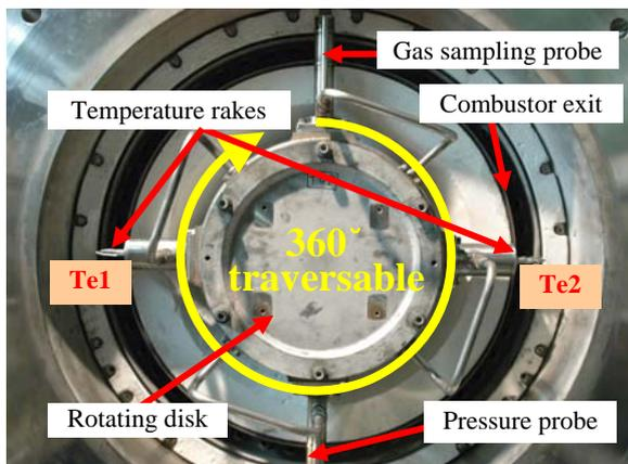
Fig.5. Temperature rakes Te1 and Te2, gas and pressure sampling probes traversable at combustor exit.
