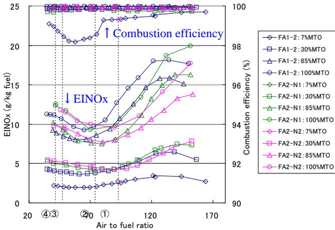
Fig.6. Emission characteristics of FA1-2 and FA2-N1 under LTO cycle conditions.
