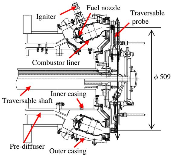
Fig.4. Schematic drawing of full annular combustor with traversable measurement system.
