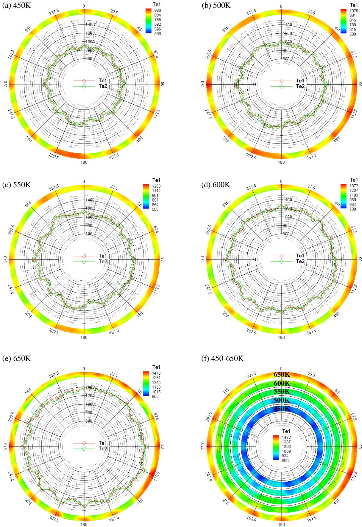
Fig.10. 2D-distributions of exit temperature Te1 and circumferential profiles of Te1 and Te2 of FA2 under parametric test conditions.
