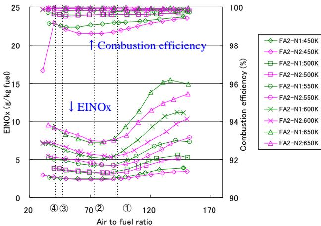
Fig.7. Emission characteristics of FA2-N1 and FA2-N2 under parametric test conditions.
