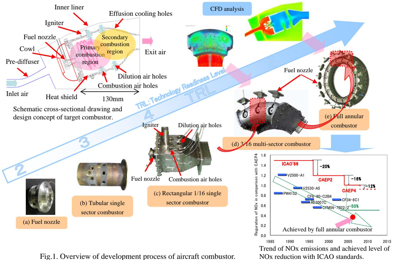
Fig.1. Overview of development process of aircraft combustor.
