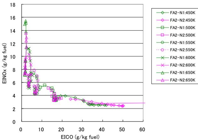
Fig.8. Correlation of CO-NOx emissions of FA2-N1 and FA2-N2 under parametric test conditions.
