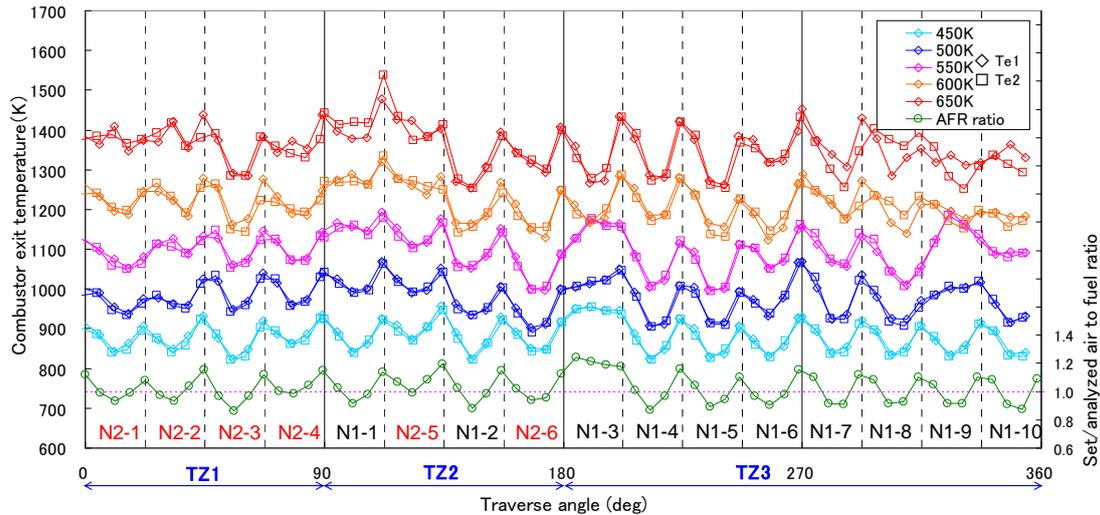
Fig.9. Circumferential profiles of temperature and AFR ratio at combustor exit of FA2 under parametric test conditions, shown with traverse zones and fuel nozzle allocation.
