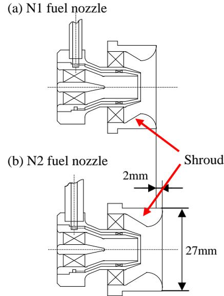
Fig.2. Difference between fuel nozzles N1 and N2.
