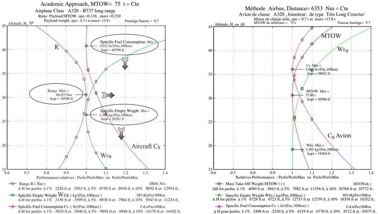
**Fig. 4** On the left, the optimum of the range  $R$ , the specific fuel consumption  $\widehat{W}_{fuel}$  and specific empty weight  $\widehat{MVOE}$  for a single-aisle type aircraft with the ACADEMIC APPROACH. And on the right, the optimum of the weight  $MTOW$ , the specific fuel consumption  $\widehat{W}_{fuel}$  and specific empty weight  $\widehat{MVOE}$  for the same type of aircraft with the MANUFACTURER APPROACH.
