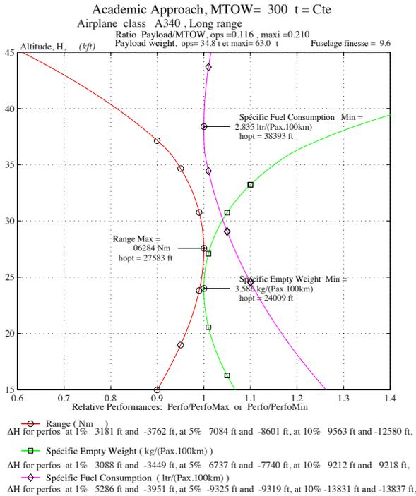
**Fig. 2** Specific Performances of an A330 or B777 Airplane Class as a function of altitude. A conceptual optimal cruise altitude exists.
