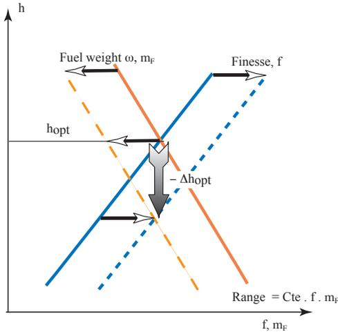
**Fig. 3** Effect of cruise speed on the conceptual optimal cruise altitude
