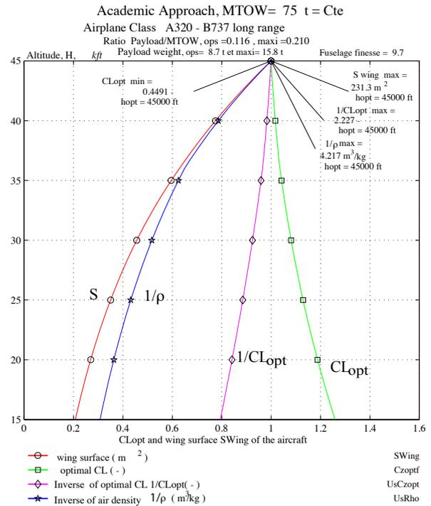
**Fig. 1** Evolution of the wing area and  $CL_{opt}$  with the altitude. It must be noted that on  $x$  abscissa axis of this figure each parameter has been divided by its minimum or maximum value.
