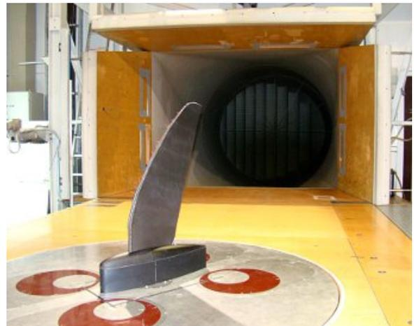
Fig. 6 Morphing model in the wind tunnel (intermediate configuration)
