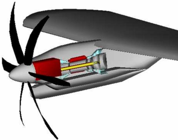
Fig. 2. PrADO Turboprop Engine Model
