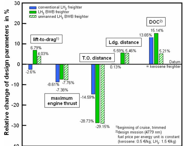
Fig. 11. Relative Comparison of Hydrogen Aircraft Versions and Reference Kerosene Aircraft
