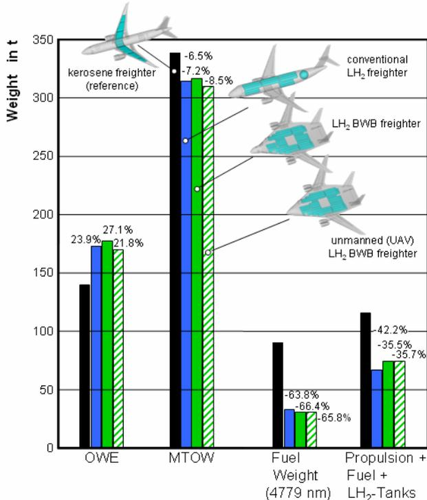
Fig. 10. Mass Comparison of Hydrogen Aircraft Versions and Reference Kerosene Aircraft
