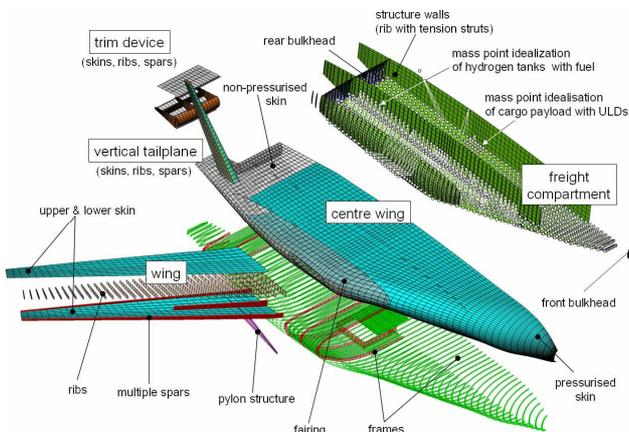
Fig. 3. PrADO SAM-Model for Structural Sizing and Mass Calculation
