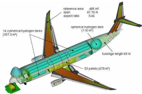
Fig. 7. Optimized Conventional Hydrogen Freighter
