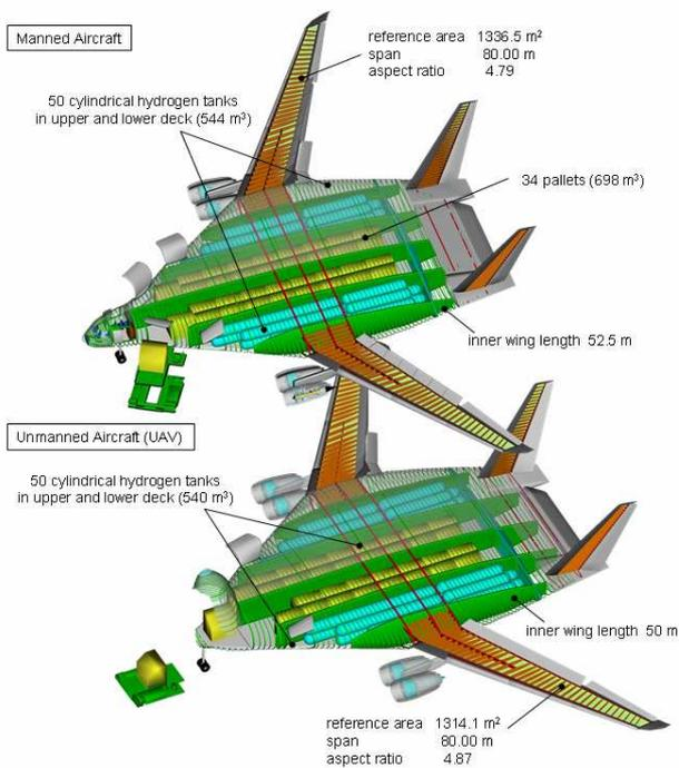
Fig. 9. Optimized Hydrogen Fueled BWB Configurations Designed for the Reference Mission of the Kerosene-Powered Freighter
