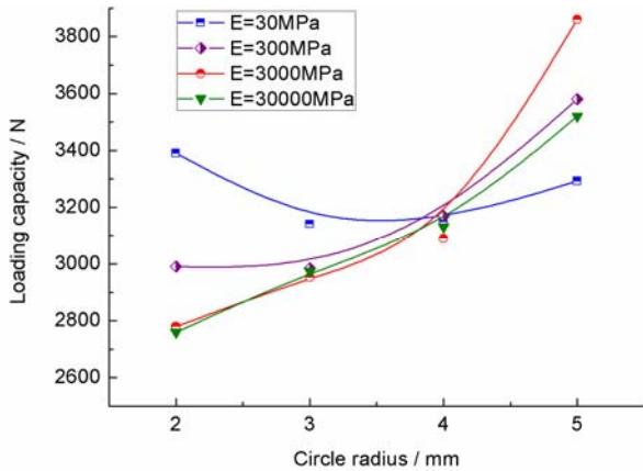
Fig.12. Loading capacity changes with the radius and stiffness of filler
