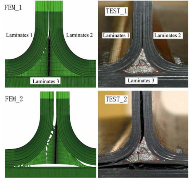
Fig.8. Failure mode of Composite T-joint under pull-off load
