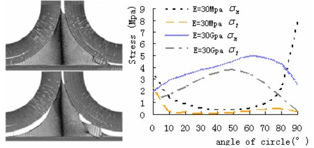
Fig. 13. The failure mode and stress distribution at the brim of filler
