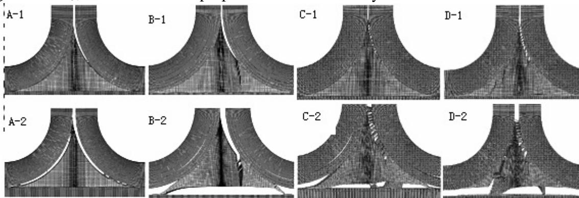
The strength and critical strain energy release rate of matrix and adhesive are reduced to 60% in A, and 80% in B, filler keeps constant; The strength and critical strain energy release rate of filler are reduced to 80% in C , and 60% in D, matrix and adhesive keep constant
