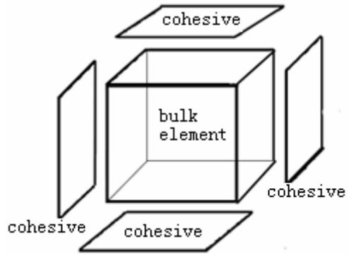
Fig. 5. Bulk element surrounded by cohesive elements
