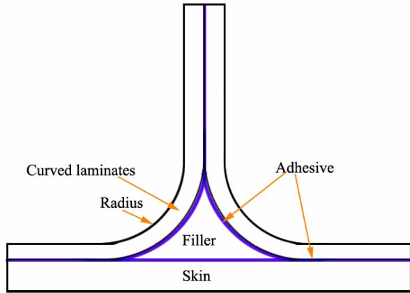
Fig.1 The geometry of T-joints
