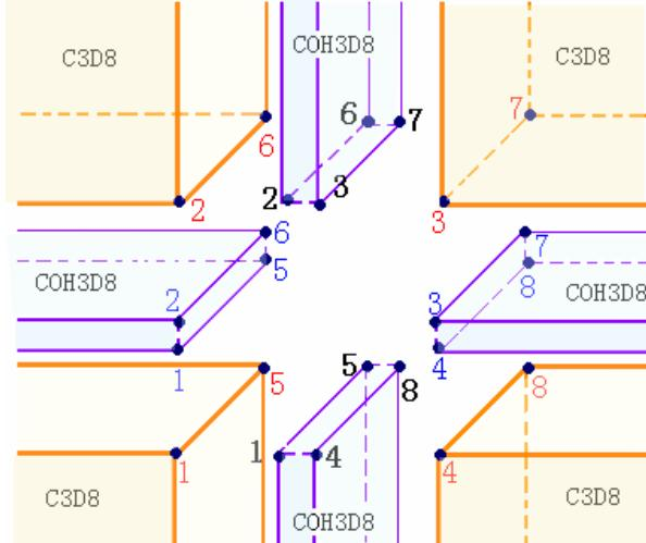
Fig.6. Nodes distribution of cohesive and bulk elements
