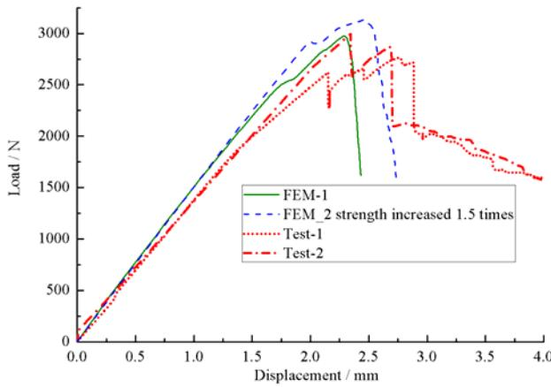
Fig.7.Load-displacement curve of composite T-joint
