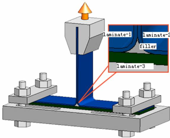
Fig.3. Sample geometry and test configuration
