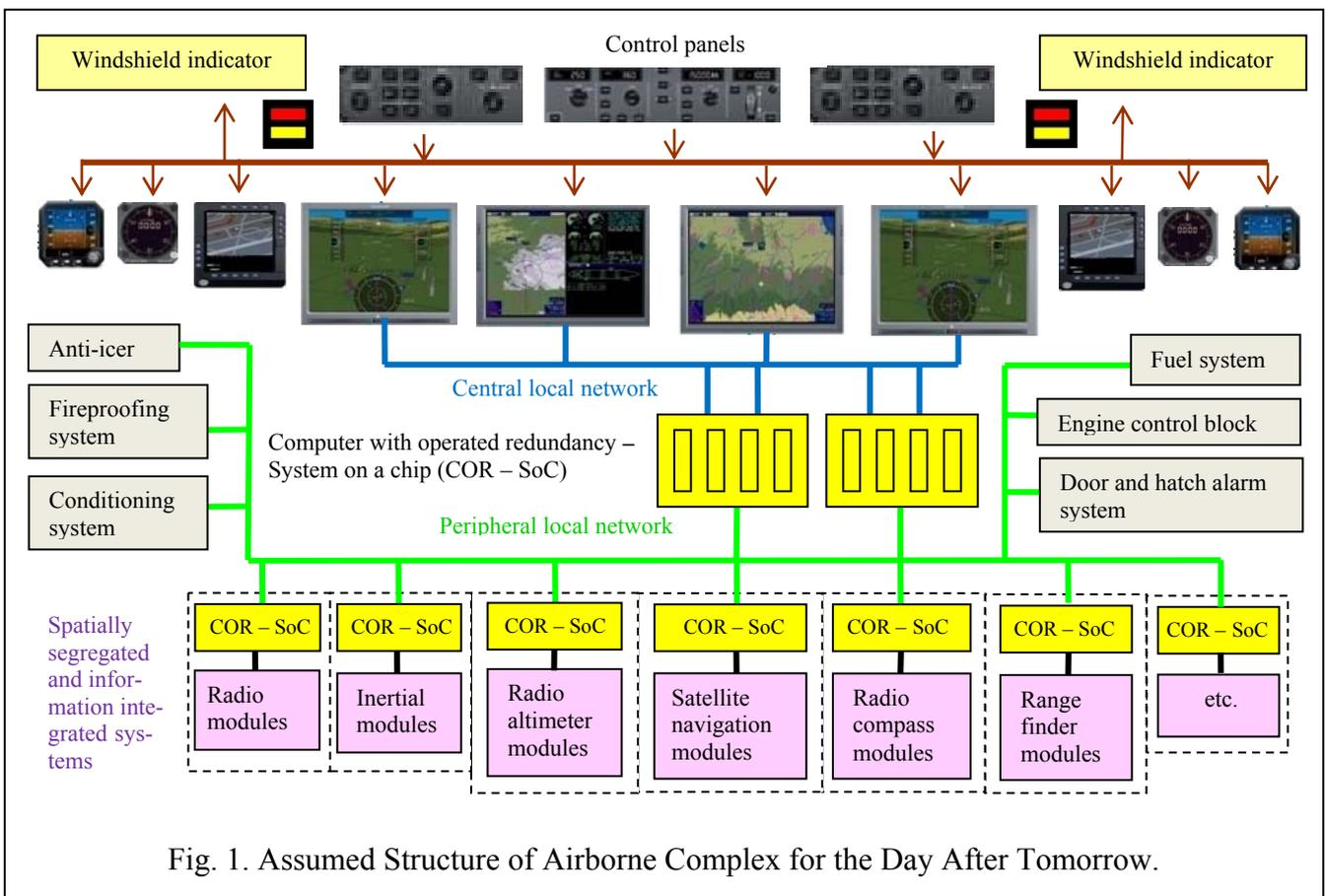
Fig. 1. Assumed Structure of Airborne Complex for the Day After Tomorrow.
