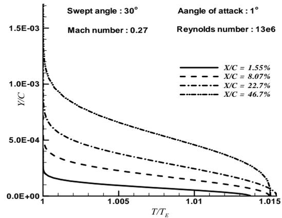
Fig.4. Computed temperature profiles  $T/T_e$  for  $M_\infty=0.27$  at various  $X/C$  stations.
