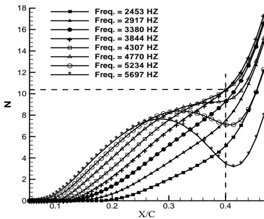
Fig. 6. Variation of the amplification factors for the frequencies of Fig.5.
