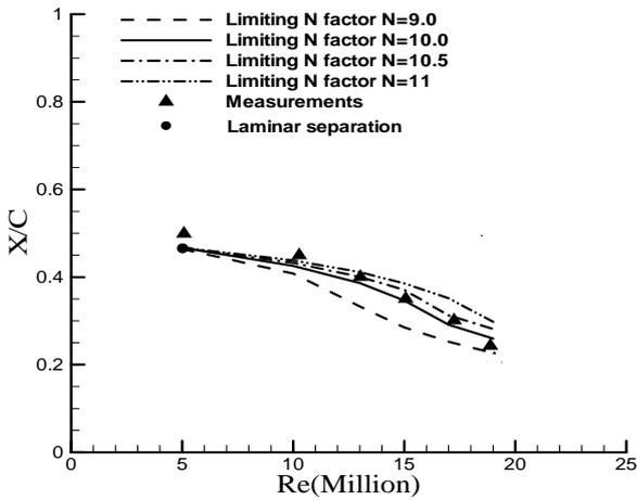
Fig. 9. Measured and computed transition locations on the upper surface of the infinite swept-wing with  $\lambda=30^\circ$  at angle of attack  $1^\circ$ .
