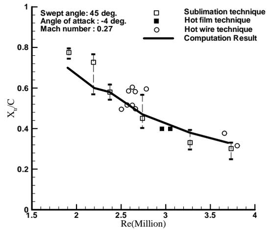
Fig. 11. The comparison between the computed transition position with the limiting  $N_{limit}$  factor as 12.1 and the measured transition position on the upper surface of the infinite swept wing model with the NLF(2)-0415 profile.
