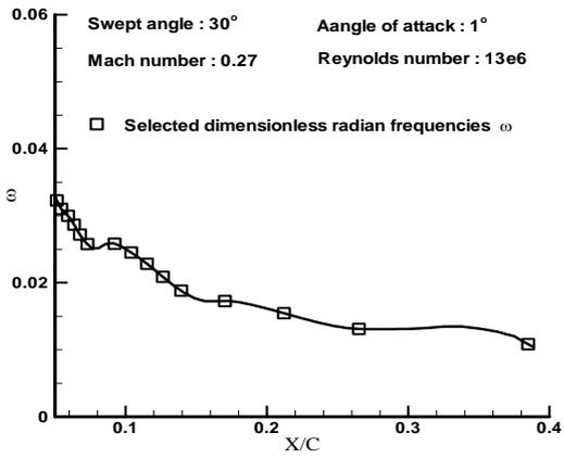
Fig. 5. Variation of  $\omega$  on zarf for  $M_\infty=0.27$  on the upper surface of the infinite swept wing model.
