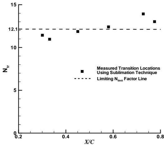
Fig. 10.  $N_{tr}$ - $X/C$  diagram on the surface of the infinite swept wing model with the NLF(2)-0415 profile.
