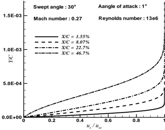
Fig. 2. Computed streamwise velocity profiles  $u_s/u_{se}$  for  $M_\infty=0.27$  at various  $X/C$  stations.
