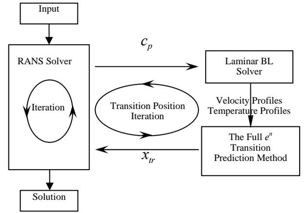
Fig.1 Sketch of the coupling the RANS solver with the transition prediction method
