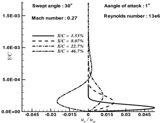
Fig. 3. Computed streamwise velocity profiles  $u_n/u_{se}$  for  $M_\infty=0.27$  at various  $X/C$  stations.
