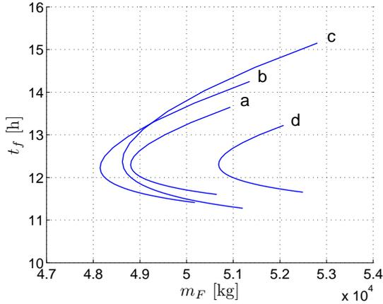
**Fig. 8** Optimal flight time vs. optimal fuel consumption, for various values of  $h_A$ : (a) 9000, (b) 10000, (c) 11000, (d) 12000 m (on each curve, the cost index ranges from  $-0.7$  to  $2$  kg/s).
