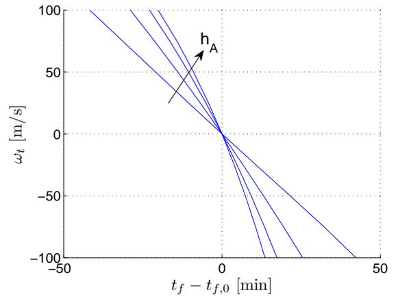
**Fig. 10** Parameter  $\omega_t$  vs. flight time ( $h_A = 9000, 10000, 11000, 12000$  m).
