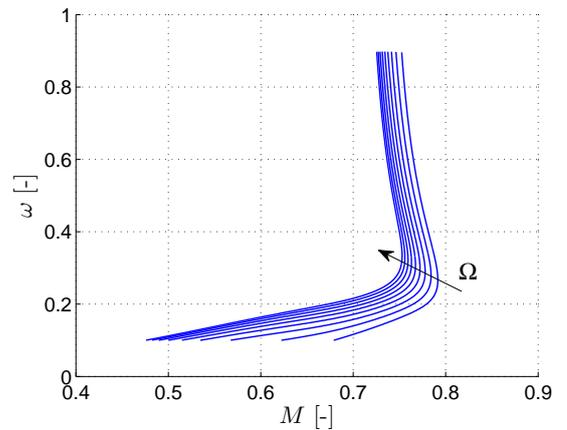
**Fig. 5** Singular arcs in the  $(\omega, M)$ -plane, for  $h_A = 10000$  m ( $\Omega = -100, -75, -50, -25, 0, 25, 50, 75, 100$  m/s).
