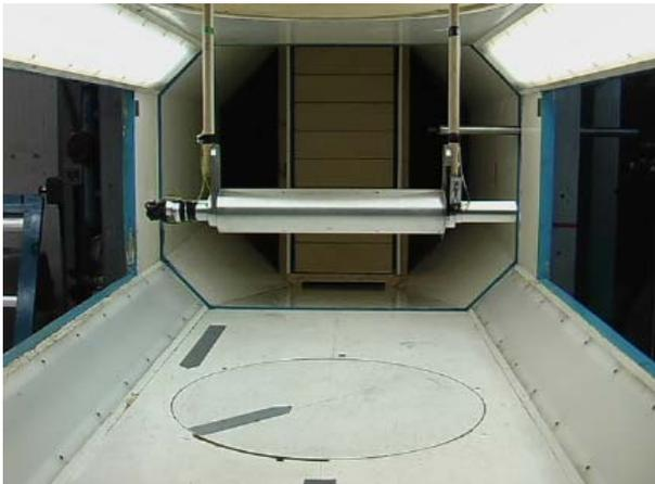
Fig. 2 Cylinder installed in the low-speed wind tunnel [3] at City University London
