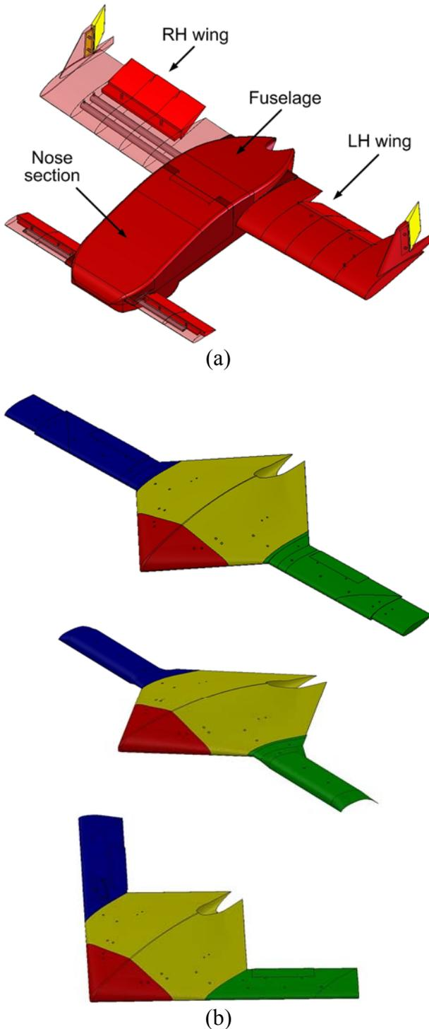
Fig. 7. CAD models of (a) “Flying-car”, and (b) MORPHEUS with the interchangeable wings, showing the four main parts of the wind tunnel models: fuselage, nose section and two wings
