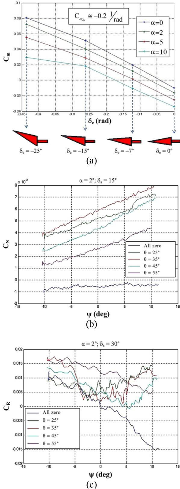
Fig. 6. CERBERUS testing results: (a) the elevons' influence, (b) the yawing-moment coefficient vs. yaw angle, and (c) spoiler's influence on roll for different hinge angles with  $2^\circ$  angle of attack and  $30^\circ$  spoiler opening
