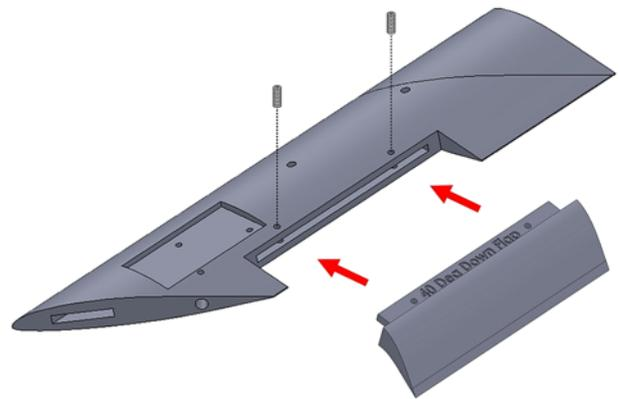
Fig. 11. Detail of an elevon and wing showing the locating features and the fastening by screws. An inscription made as part of the RP process contains the elevon's designation
