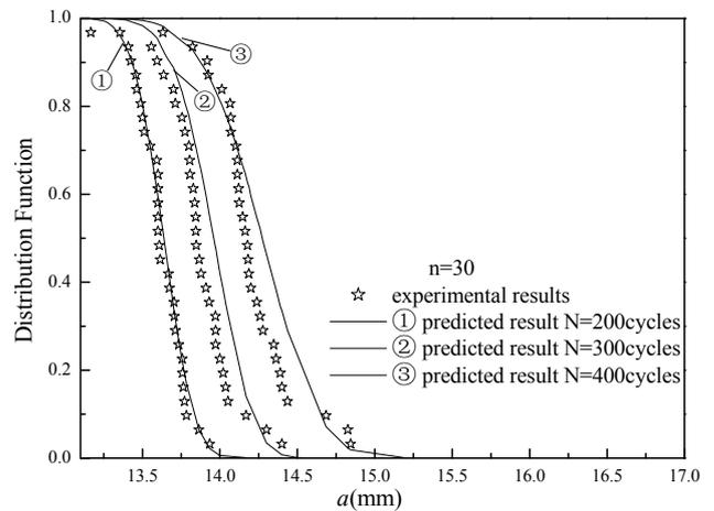
**Fig.5 Crack size distribution at a given load cycle**
