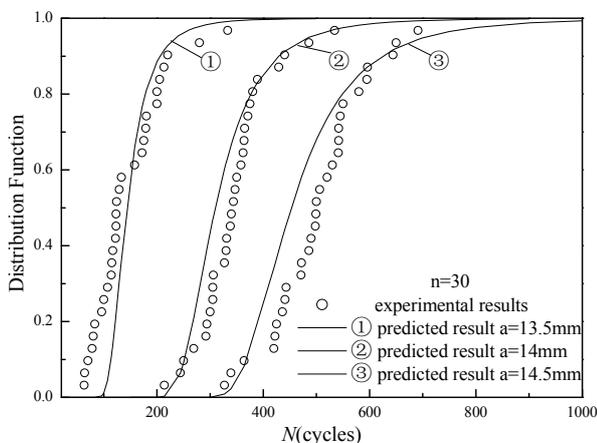
**Fig.4 Number of load cycles distribution to reach the specified crack sizes**
