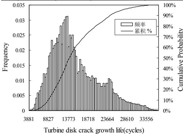
**Fig.9 The cumulative density function of crack growth life for turbine disk**
