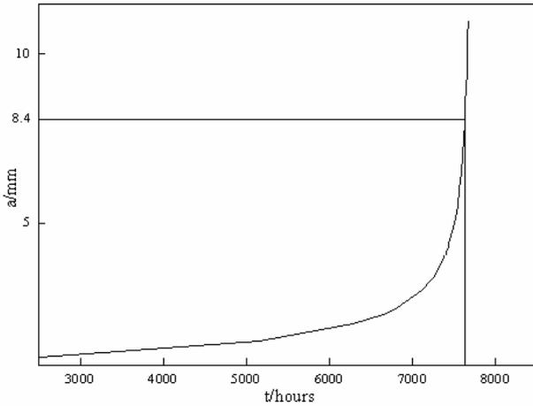
Fig.8 The relationship between flight time to crack size
