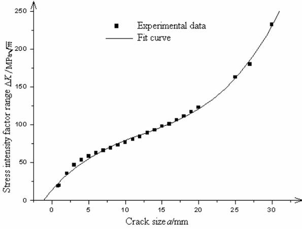
Fig.7 The curve of  $\Delta K - a$
