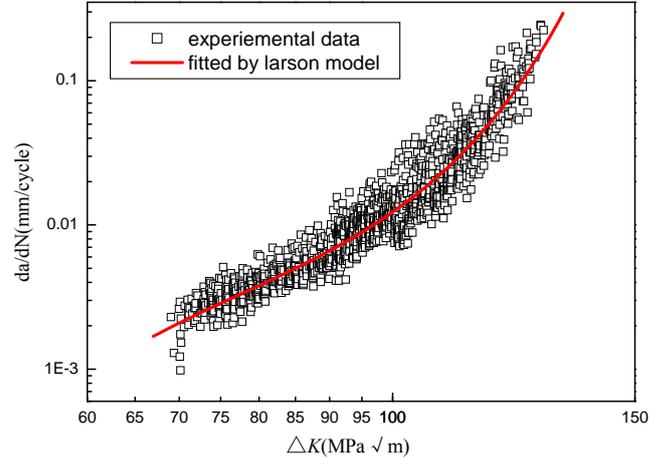
**Fig.3 Median FCCG curve**
