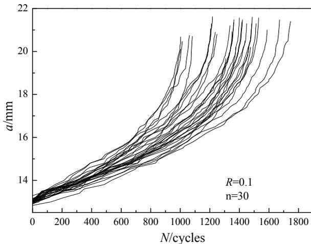
**Fig.2 Experimental FCCG curves for GH4133B**
