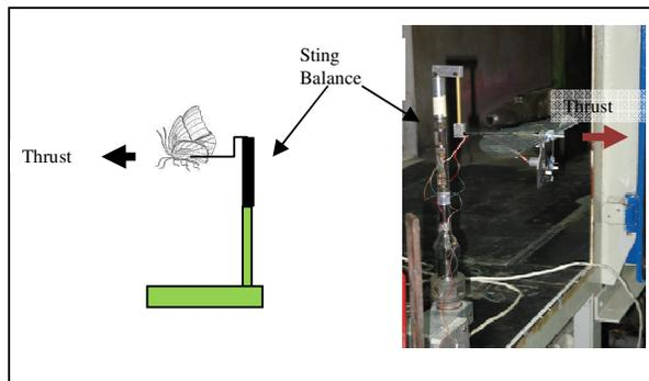
Fig. 11. Sting balance and model
