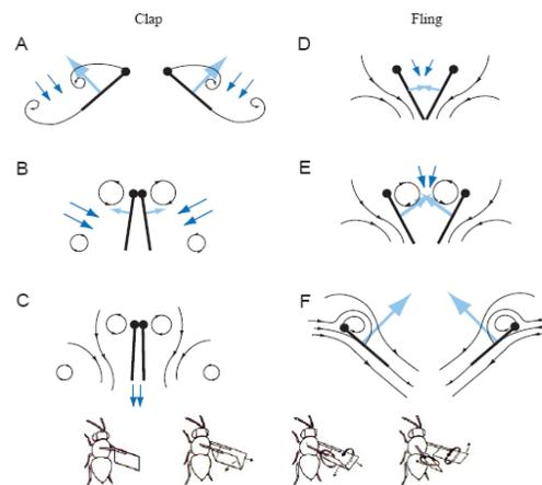
Fig. 2. "Clap & Fling" affect - process scheme.
