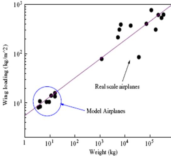
Fig. 4. Wing Loading Vs. Weight (Airplanes)
