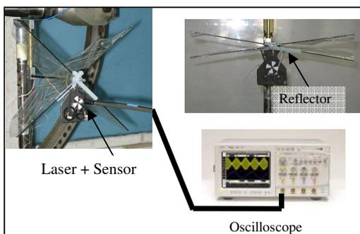
Fig. 12 Frequency measurement
