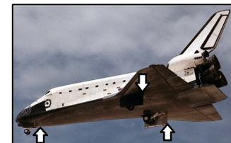
considered as a higher risk than the reutilization of airframe. A shuttle is operated based on a design concept of reutilizing everything in the orbiter. Main wings, gaining a lifting force at the time of flying as a fixed-wing airplane after atmosphere re-entry, are the parts with the largest area in the orbiter and integrated with the airframe bottom as one of the most heat-exposed areas.
