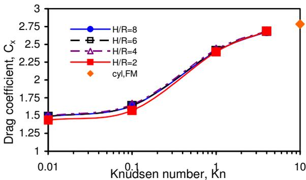
Fig. 7. Drag coefficient  $C_x$  of a torus vs. Knudsen number  $Kn_{\infty,D}$  and various geometrical factors  $H/R$  in the flow of nitrogen at  $M_{\infty} = 10$ .
