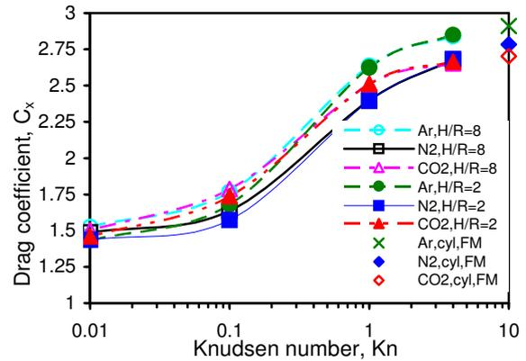
Fig. 8. Drag coefficient  $C_x$  of a torus vs. Knudsen number  $Kn_{\infty,D}$  and various geometrical factors  $H/R$  in argon, nitrogen, and carbon dioxide at  $M_{\infty} = 10$ .
