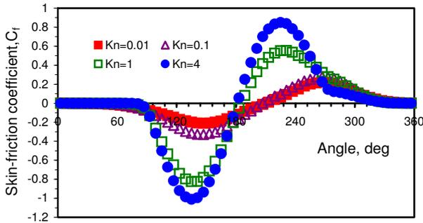
Fig. 6. Skin-friction coefficient  $C_f$  along the torus surface in nitrogen flow at  $H/R = 2$ ,  $M_{\infty} = 10$ , and various Knudsen numbers  $Kn_{\infty,D}$ .
