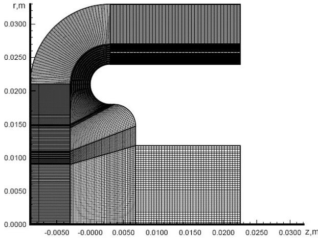
Fig. 10. The grid near the model used in simulations.
