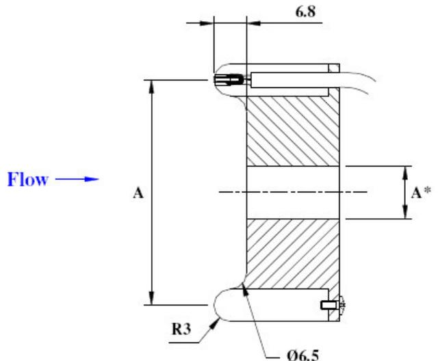
Fig. 9. The ballute model used in experiments [17].
