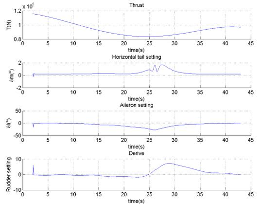
Fig. 2.2 Input history during optimized trajectory
