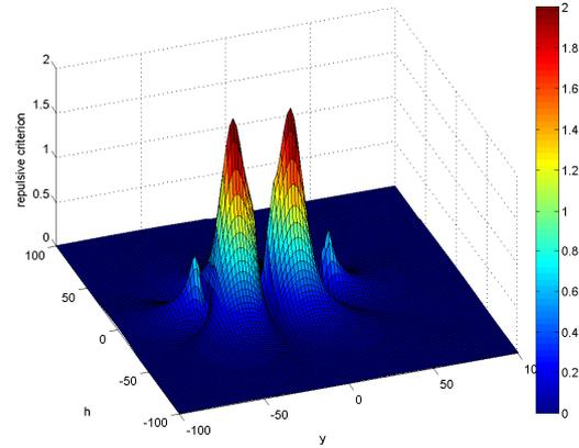
Fig. 3: Repulsive potential in a plane orthogonal to aircraft trajectory
