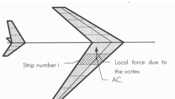
Fig 1. Principles of the strip theory method
