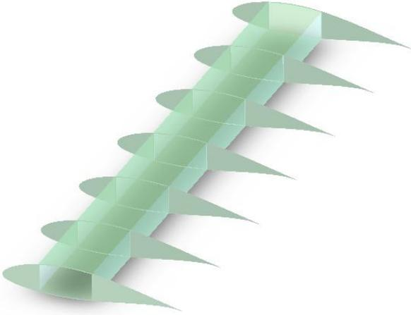
**Fig. 1** Proposed spar-tank configuration.
