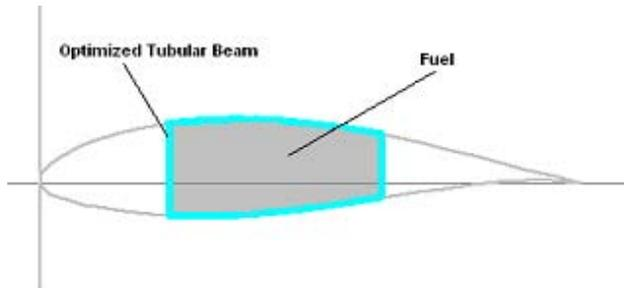
**Fig. 2** Cross section of the wing.
