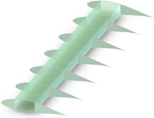
**Fig. 1** Proposed spar-tank configuration.
