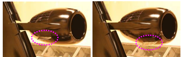
Figure 12. Chine installation in the experiment.
