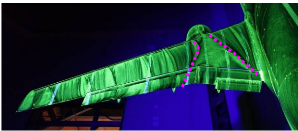
Figure 5. Surface flow pattern at post-stall conditions for the long-cowling nacelle. ( V = 60m/s , AoA=15deg )
